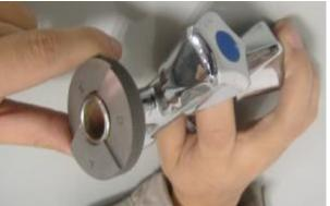
**Determine** 判断: You can't turn more even by small force (No distortion) .This status means the matched threads already at the end position.
