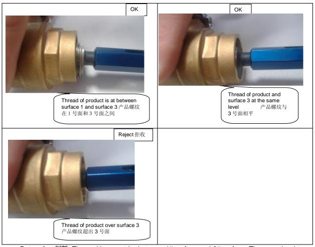
**Determine** 判断: The position must be between 1# surface and 3# surface. The same level to 3# can be accepted too, but can't be accepted if the same level to 1# surface.
