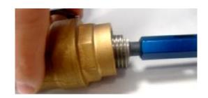
**Determine** 判断: You can't turn more even by small force (No distortion) .This status means the fitting threads already at the end position.
